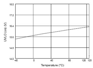
Fig. 1 UVLO (on) vs. Temperature
