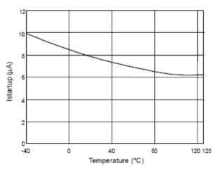
Fig. 9 Startup Current (Istartup) vs. Temperature
