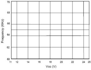
Fig. 5 Frequency vs. Vcc
