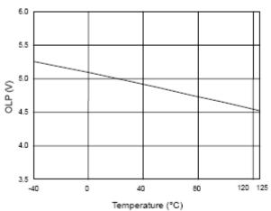
Fig. 12 OLP-Trip Level vs. Temperature
