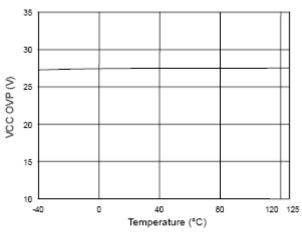
Fig. 10 VCC OVP vs. Temperature
