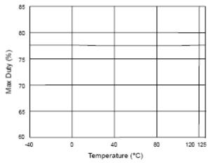
Fig. 7 Max Duty vs. Temperature
