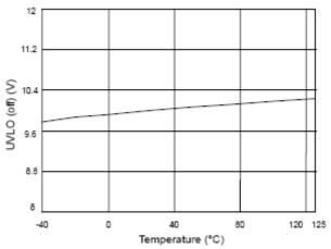
Fig. 2 UVLO (off ) vs. Temperature
