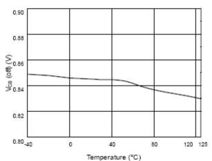
Fig. 8 V<sub>CS</sub> (off) vs. Temperature
