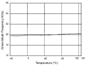
Fig. 4 Green Mode Frequency vs. Temperature
