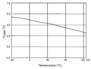
Fig. 11 V<sub>COMP</sub> open loop voltage vs. Temperature
