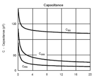
VDS - Drain-to-Source Voltage (V)
