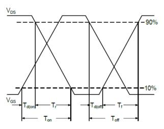
Fig.10 Switching Time Waveform
