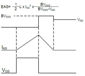
**Fig.11 Unclamping Inductive Waveform**
